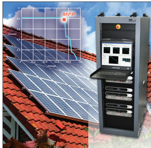
Figure 2. Solar Array Simulators, like the AMETEK Terra SAS shown here, make it possible to test solar inverters over a range of input conditions
