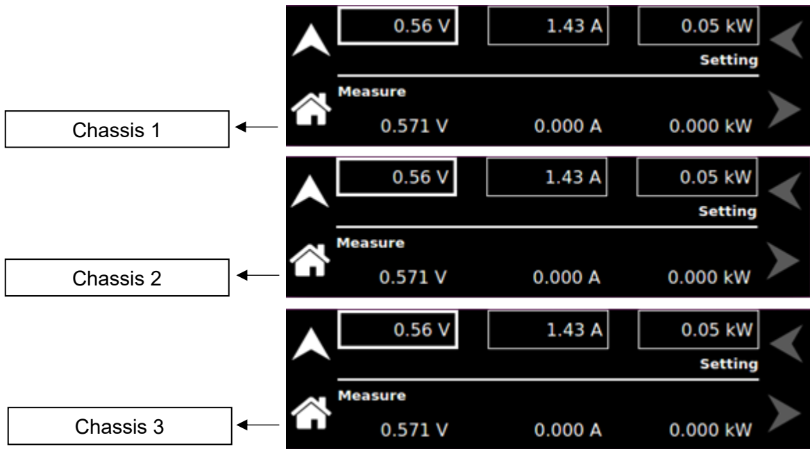
Figure 6-7: Multi-Chassis Communication Screens
