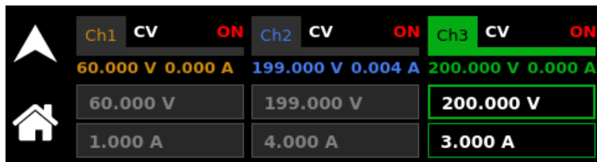
Figure 3-26: Real-Time, Immediate Output Parameter Adjustment
