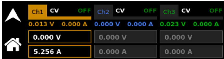
Figure 3-10: DASHBOARD Screen Current Selection-Field Active using Encoder switch
