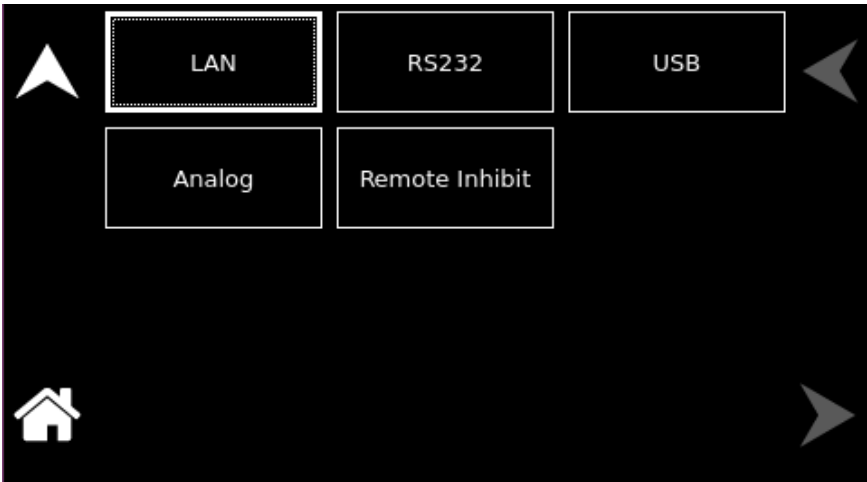
Figure 10-181. Control Interface Screen Top-Level Menu
