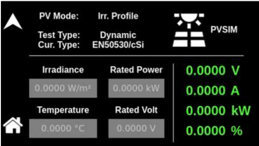
Figure 11-16. Dashboard Screen (Oper. Type – Profile, Test Type – Dynamic and Curve Type – EN50530)
