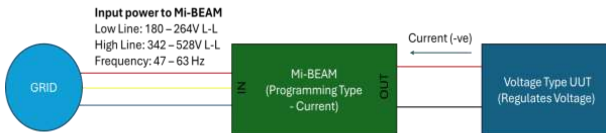
Figure 10-2. Voltage Type UUT
