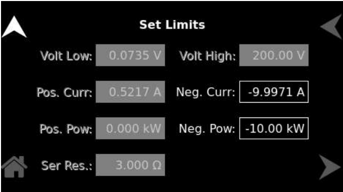
Figure 10-62. Set Limits – CV/CC, CV/CP and CV
