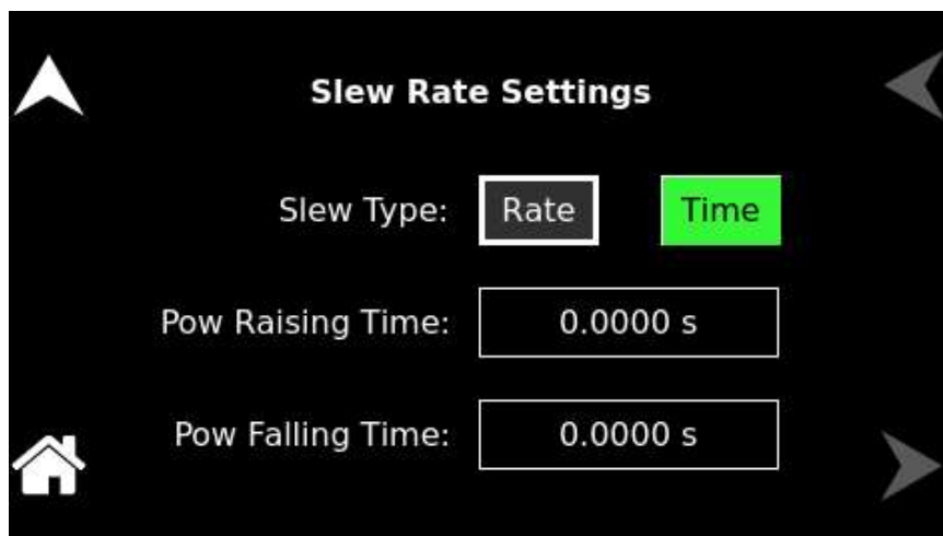
Figure 9-92. Slew Rate Settings – Power (CP/CC)
