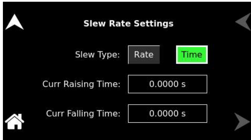
Figure 9-91. Slew Rate Settings – Current (CC/CV, CC/CP and CC)
