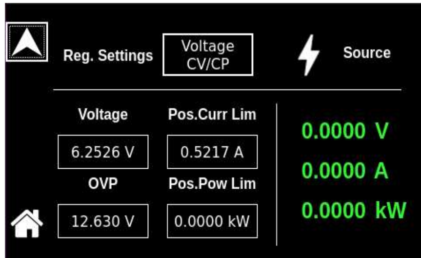
Figure 9-7. Dashboard Screen in Voltage CV/CP Regulation setting
