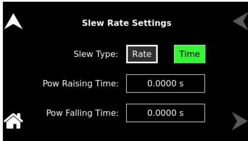
Figure 10-100. Slew Rate Settings – Current (CP/CV)
