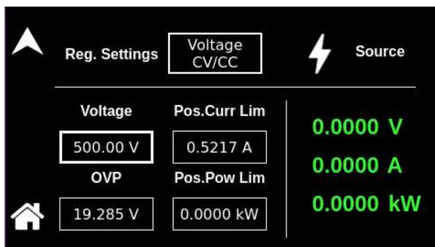
Figure 9-15. Real-Time, Immediate Output Parameter Adjustment
