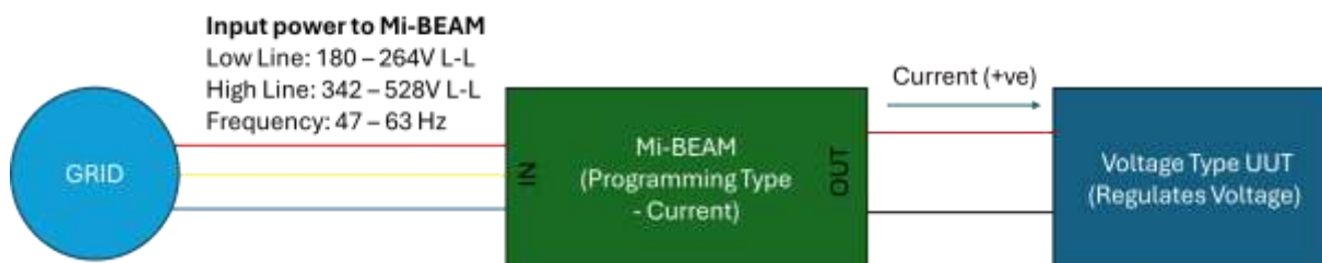
Figure 11-1. Voltage Type UUT
