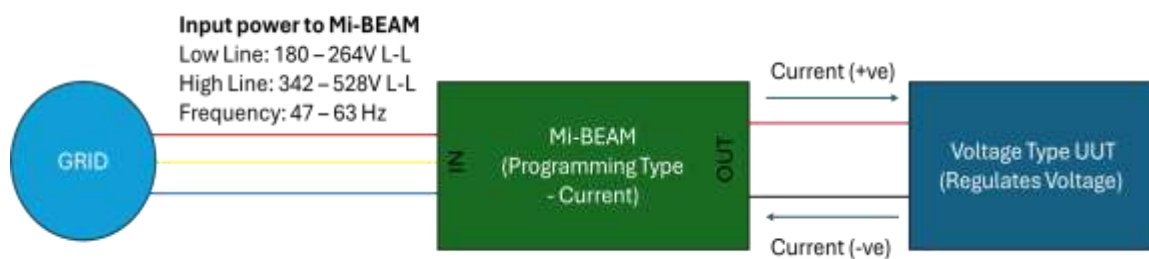
Figure 13-1. Voltage Type UUT
