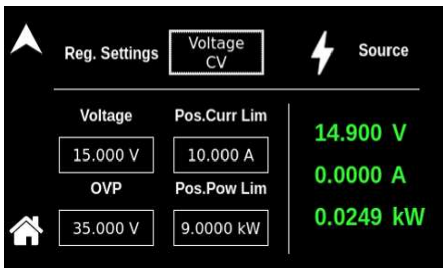
Figure 9-8. Dashboard Screen in Voltage CV Regulation setting
