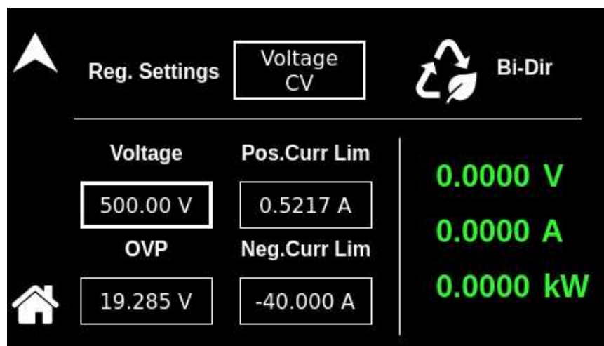
Figure 8-7. Dashboard Screen in CV Mode
