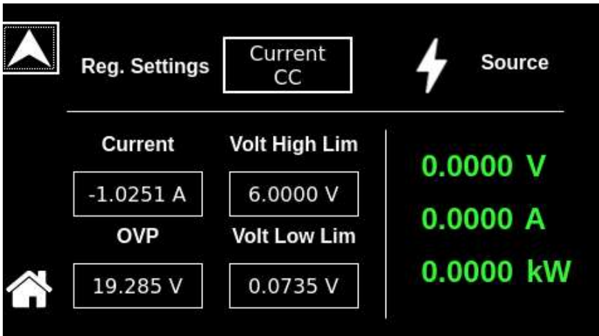
Figure 9-13. Dashboard Screen in Current CC Regulation setting
