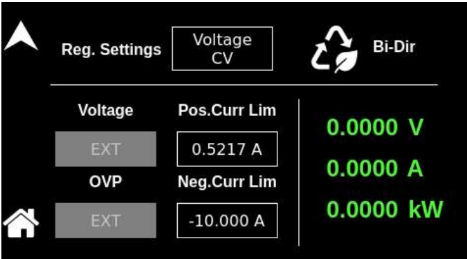
Figure 8-183. Dashboard Screen – Voltage (EXT)
