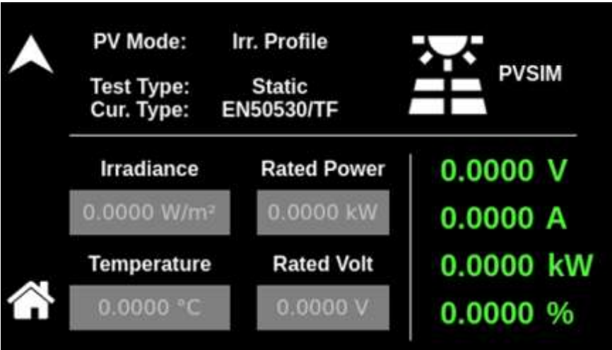
Figure 11-13. EN50530 Test Type Settings - Static
