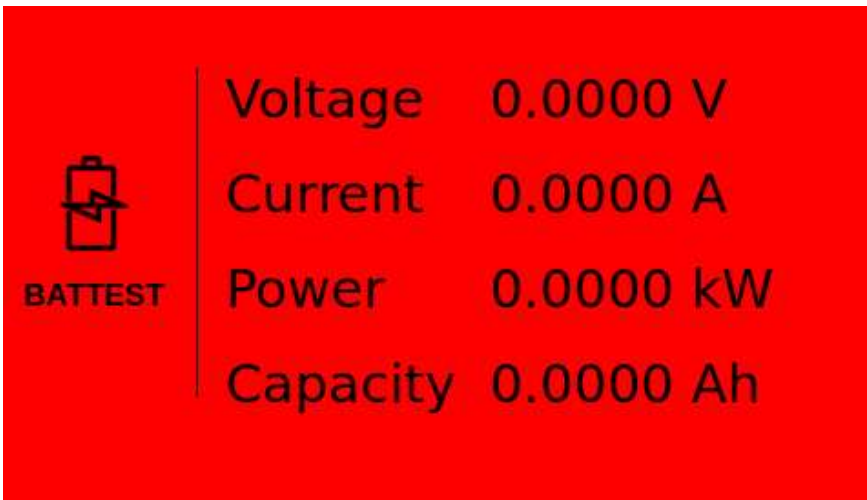
Figure 7-12. Dashboard Screen (Output State – OFF, Fault – YES and Power Direction – NA )
