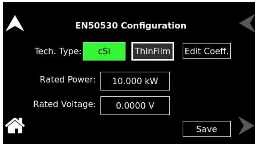
Figure 11-73. EN50530 Configuration (Tech. Type – cSi)
