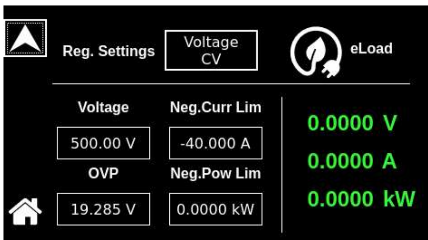
Figure 10-8. Dashboard Screen in Voltage CV Regulation setting
