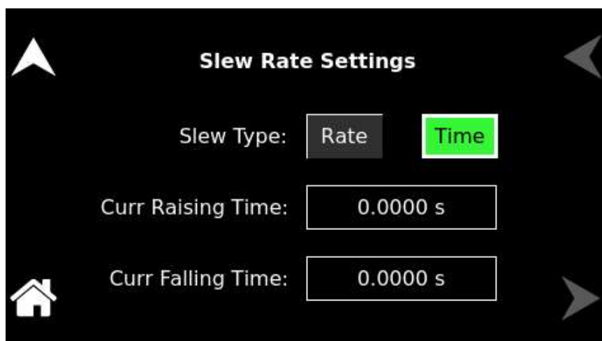
Figure 10-99. Slew Rate Settings – Current (CC/CV and CC)
