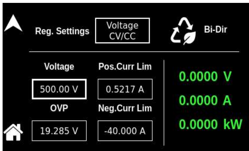
Figure 7-4. DASHBOARD Screen Menu with Voltage Selection-Field Active
