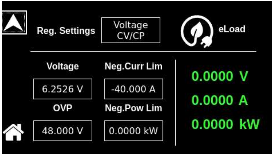
Figure 10-7. Dashboard Screen in Voltage CV/CP Regulation setting
