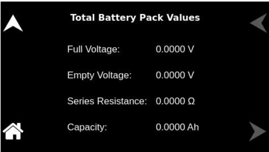
Figure 12-20. Total Battery Pack Values – Battery
