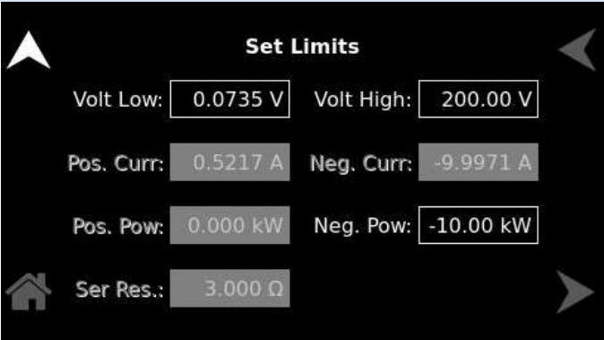
Figure 10-80. Set Limits - CC/CV, CC/CP and CC
