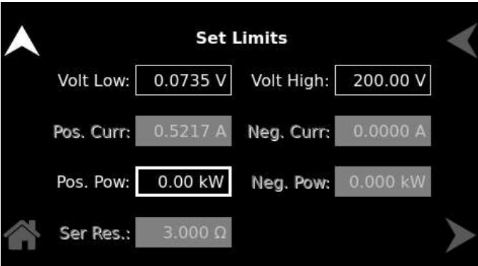
Figure 9-73. Set Limits - CC/CV, CC/CP and CC
