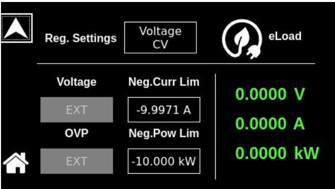
Figure 10-174. Dashboard Screen – Voltage (EXT)
