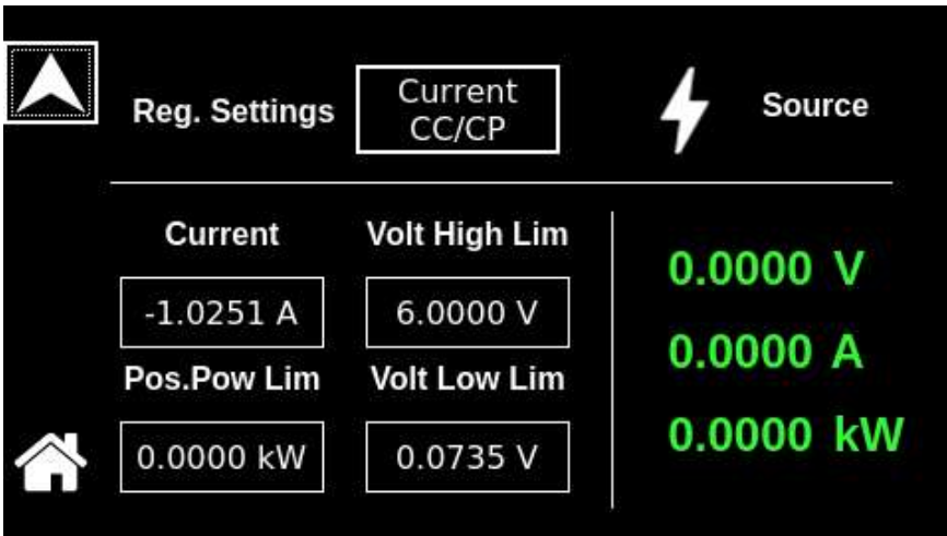
Figure 9-12. Dashboard Screen in Current CC/CP Regulation setting
