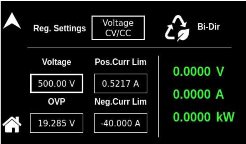
Figure 8-14. Real-Time, Immediate Output Parameter Adjustment
