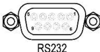
Figure 3-38. RS-232C Interface Connector
