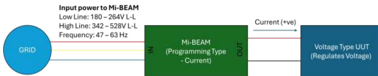
Figure 9-2. Voltage Type UUT
