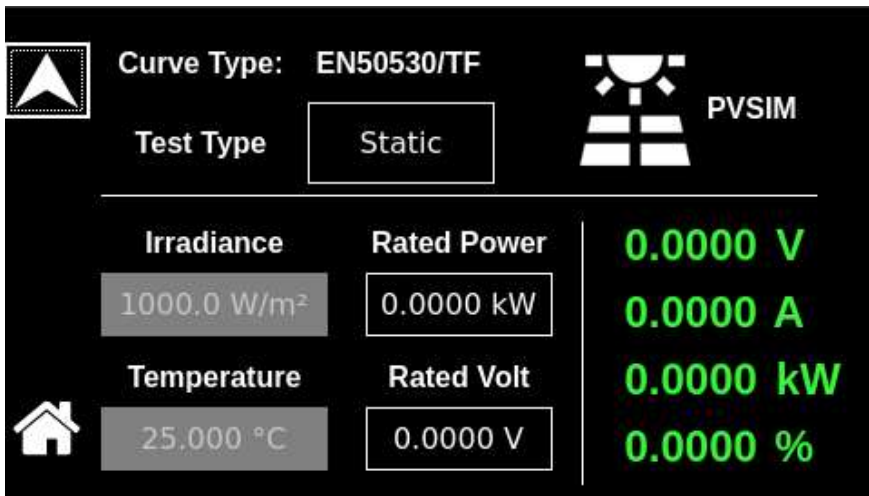
Figure 11-5. EN50530 Test Type Settings - Static
