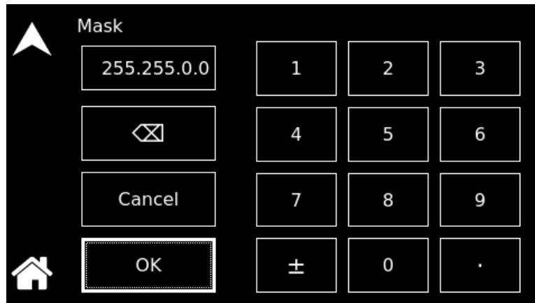
Figure 7-7. LAN Screen - Subnet Mask
