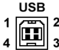
Figure 4-10: USB Connector pin orientation.
