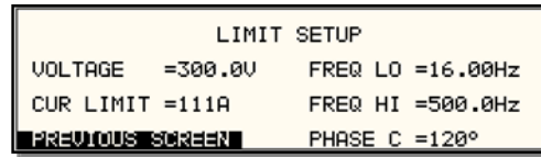
Figure 5-21: LIMIT SETUP Menu
