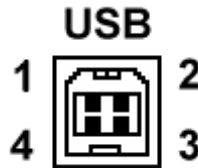
Figure 3-13: USB Connector pin orientation.
