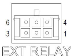
Figure 3-16. External Relay Interface Connector
