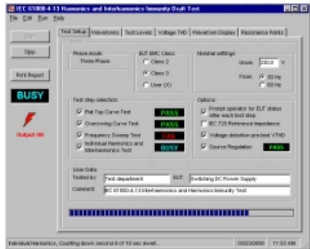
Figure 4: IEC 61000-4-13 Test Window
