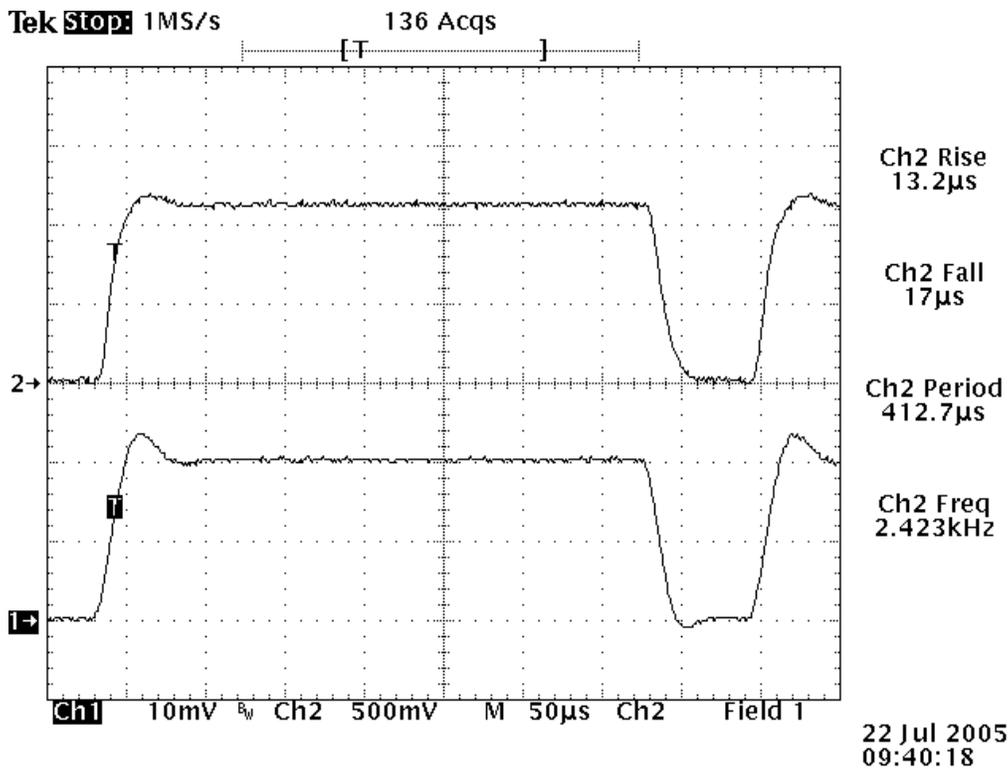
Figure 9. Current monitor output from the DC load (top); current through the diodes (bottom) while pulsing 0-40A at a 2.4 kHz repetition rate with a 20% duty cycle. Note that the current monitor tends to filter the initial overshoot due to internal circuit filtering bandwidth limitations. This needs to be checked with an external probe if high slew rates are to be used in order to not damage the laser diodes if they are being operated near their rated current.
