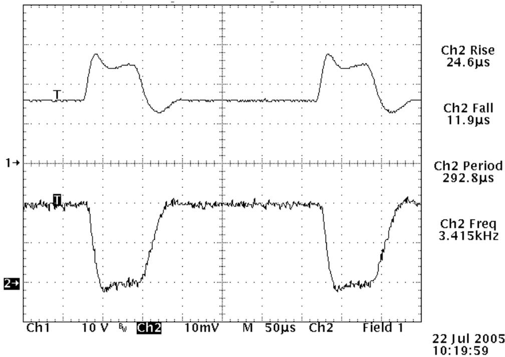
Figure 6. Voltage across to DC Load (top); current through the diodes (bottom) while pulsing 0-40A at a 3.4 kHz repetition rate with an 80% duty cycle with a medium slew rate setting. Note that no current overshoot occurs.
