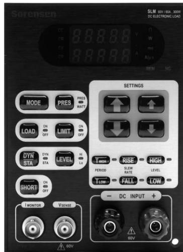
Figure 2. Front panel controller of SLH-Series Load. Full controls of slew rate are also available via GPIB or an external signal generator.
