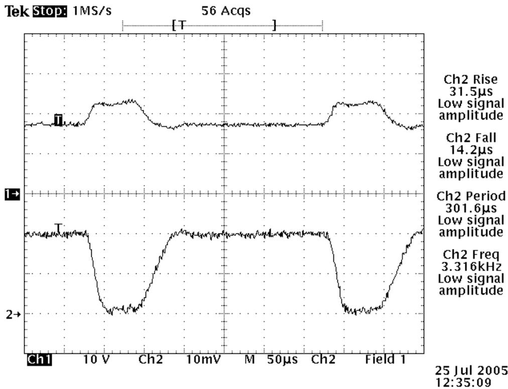
Figure 5. Voltage across to DC Load (top); current through the diodes (bottom) while pulsing 0-20A at a 3.3 kHz repetition rate with an 80% duty cycle.
