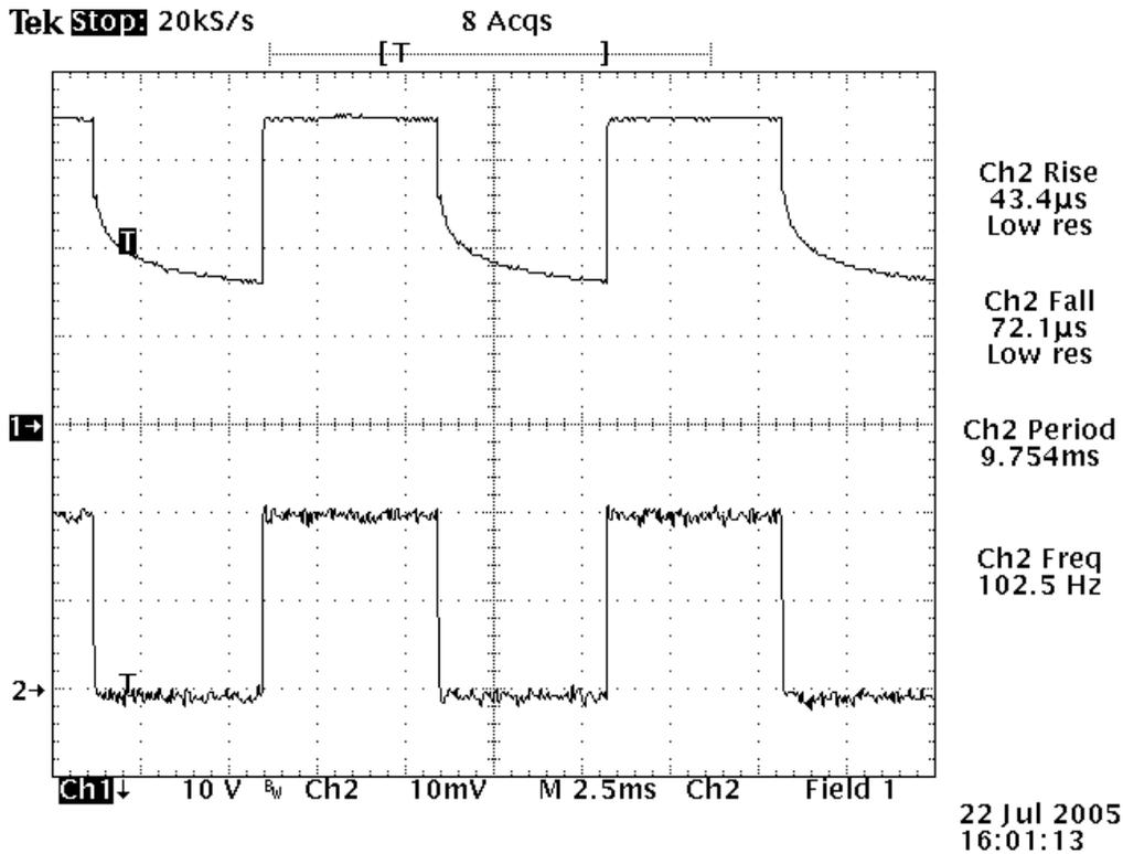
Figure 3. Voltage across the diodes (top) and the current through the diodes (bottom) while pulsing at a 102.5 Hz repetition rate with a 50% duty cycle.
