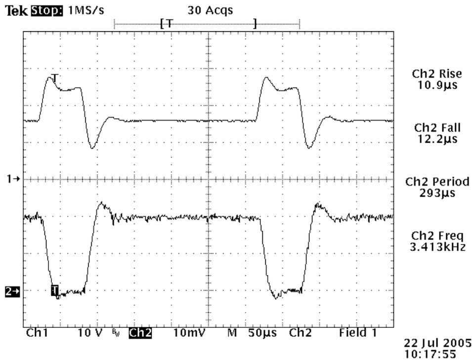
Figure 7. Voltage across to DC Load (top); current through the diodes (bottom) while pulsing 0-40A at a 3.4 kHz repetition rate with an 80% duty cycle with the slew rate set for maximum setting on the DC load. Current overshoot occurs at this slew rate due to the increased di/dt transitions. As the inductance in the cable increases, the slew rate may need to be reduced further to eliminate current overshoot.
