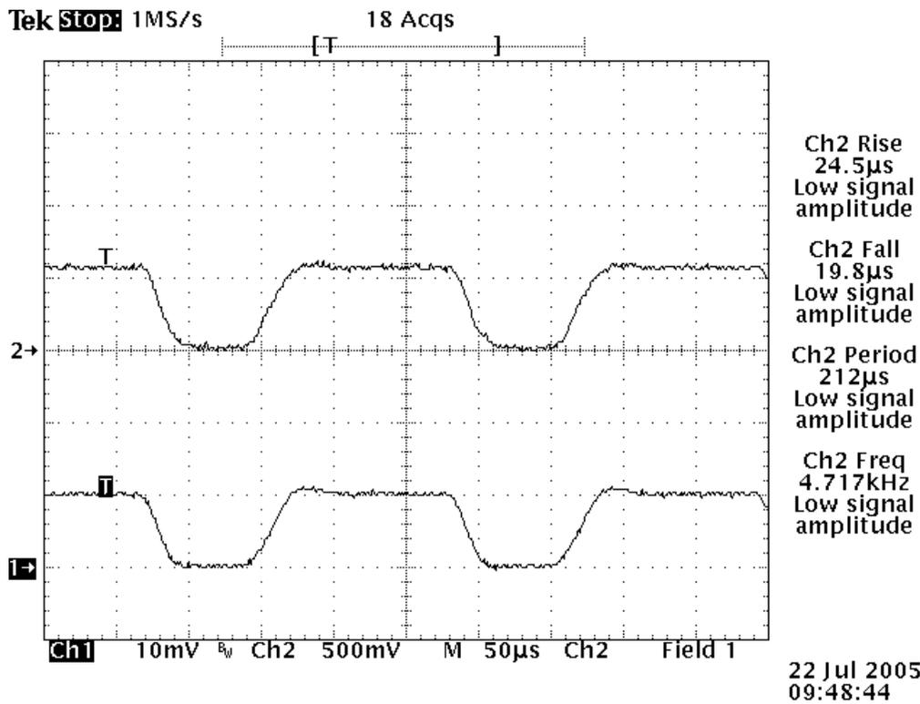
Figure 8. Current monitor output from the DC load (top) and the current through the diodes (bottom) while pulsing 0-10A at a 4.7 kHz repetition rate with a 50% duty cycle. Note that the current monitor closely resembles the waveform from the current probe.
