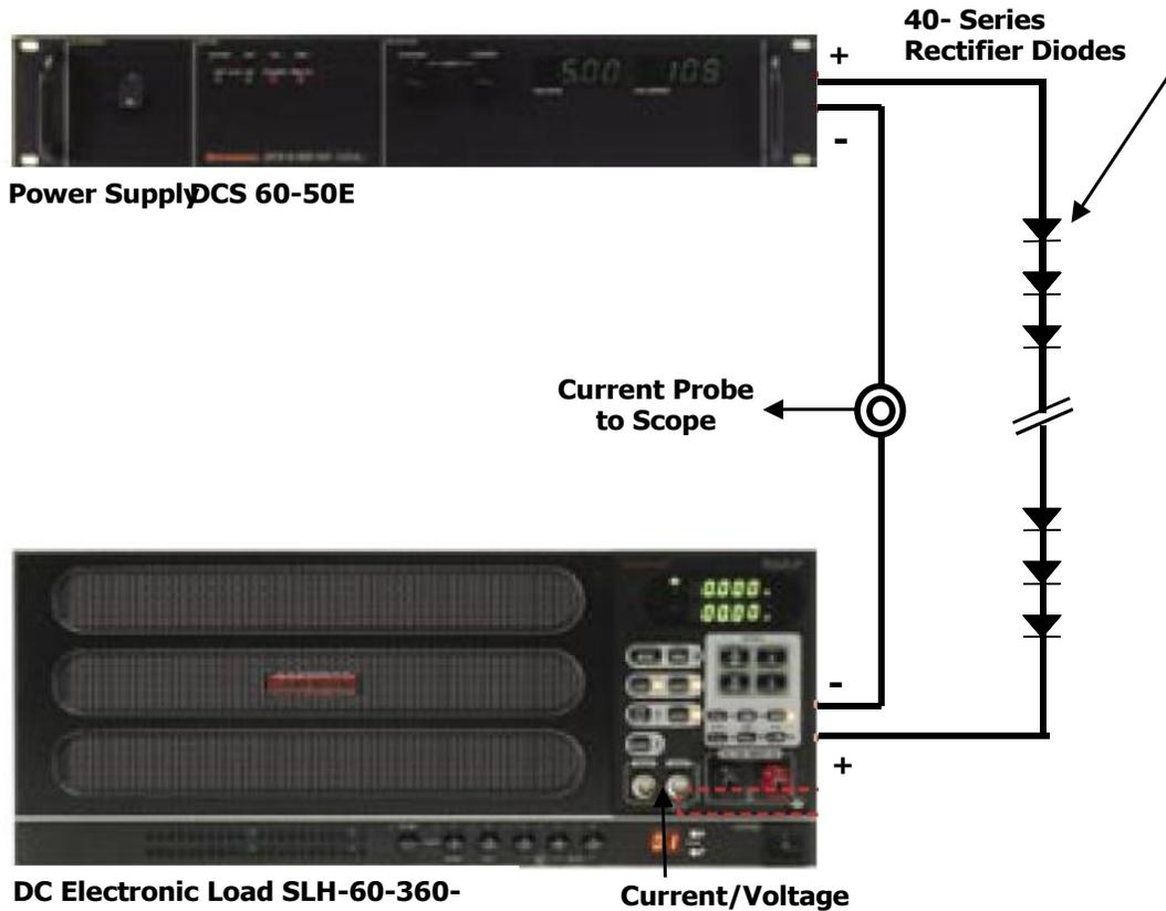
Figure 1. Diagram of DC Supply and Load with "Laser diode" Drive Scheme.
